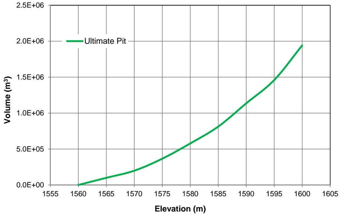
**Figure 3-7: Pit 6 Volume-Elevation Curve**
