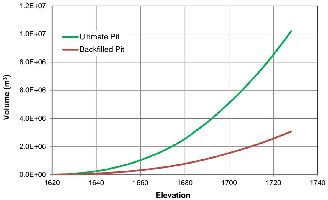
**Figure 3-9: Pit 34 Volume-Elevation Curve**
