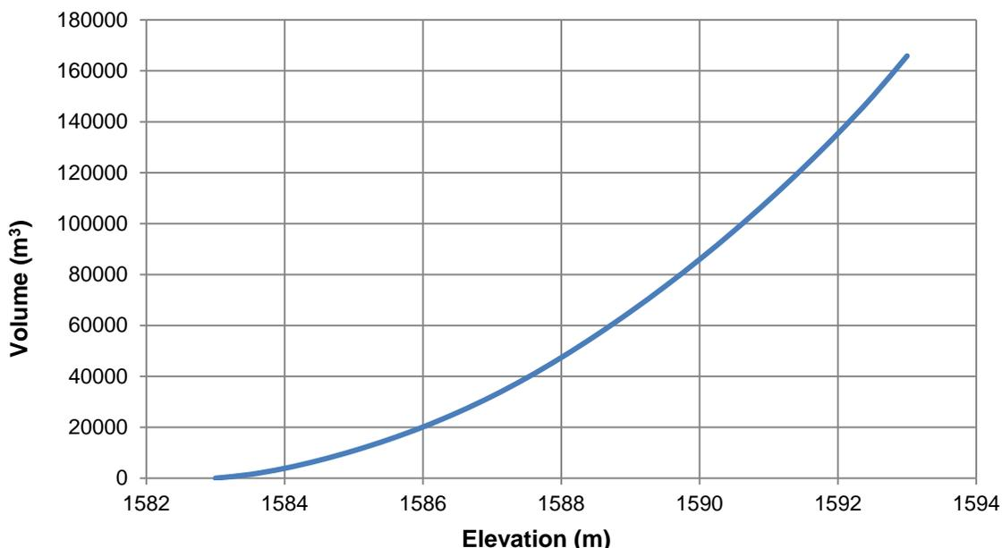
**Figure 3-5: Volume-Elevation Curve for Corbin Dam**
