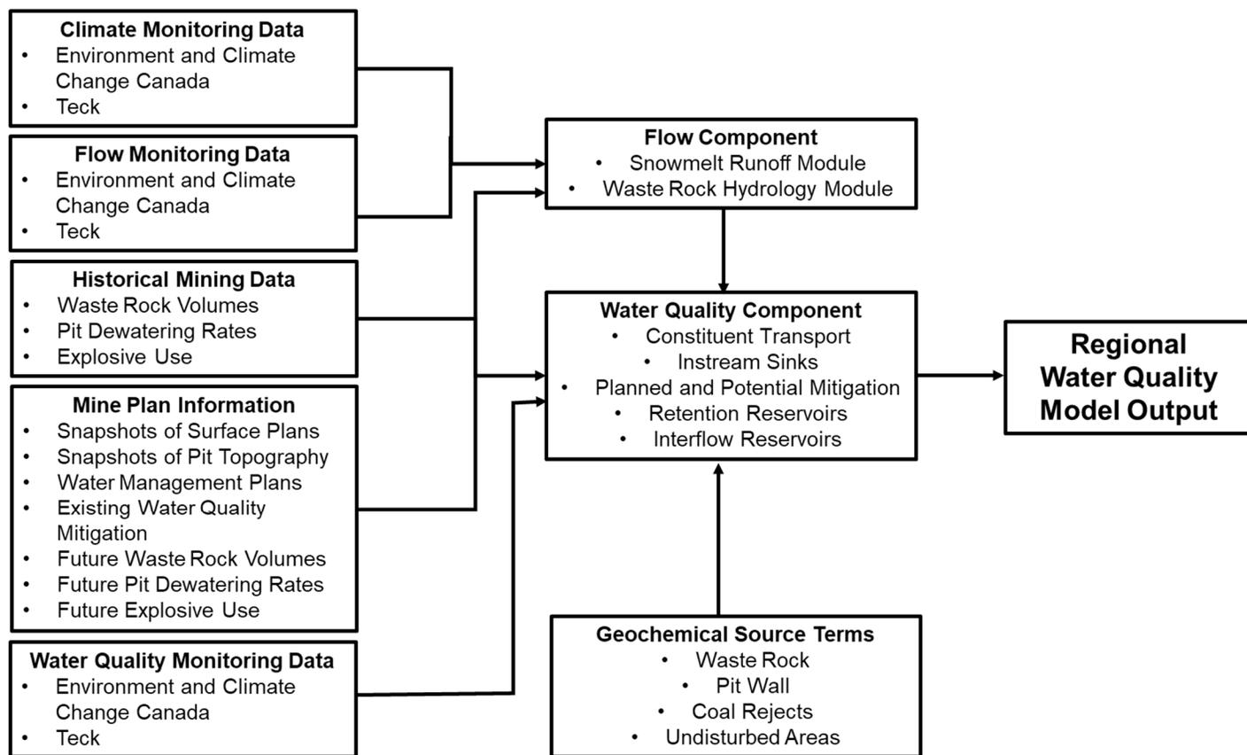
Figure 3-1: Schematic Overview of the RWQM Inputs and Components
