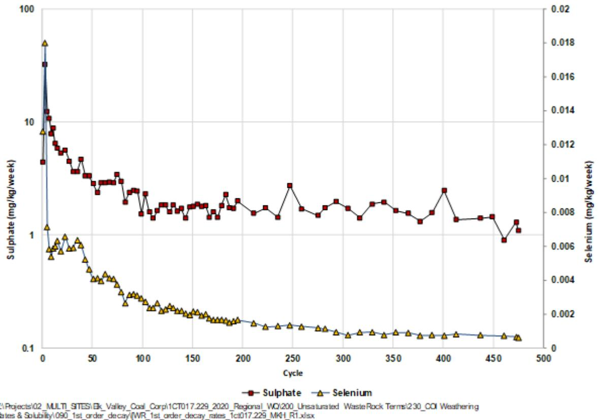
Figure 9-3: Sulphate and Selenium Release Rates for Humidity Cell (LCO HC-19) on Blasted Rock from Line Creek Operations
