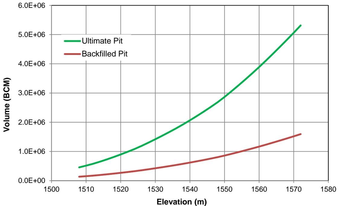
**Figure 3-8: Pit 14 Volume-Elevation Curve – Ultimate and Backfilled Pits**
