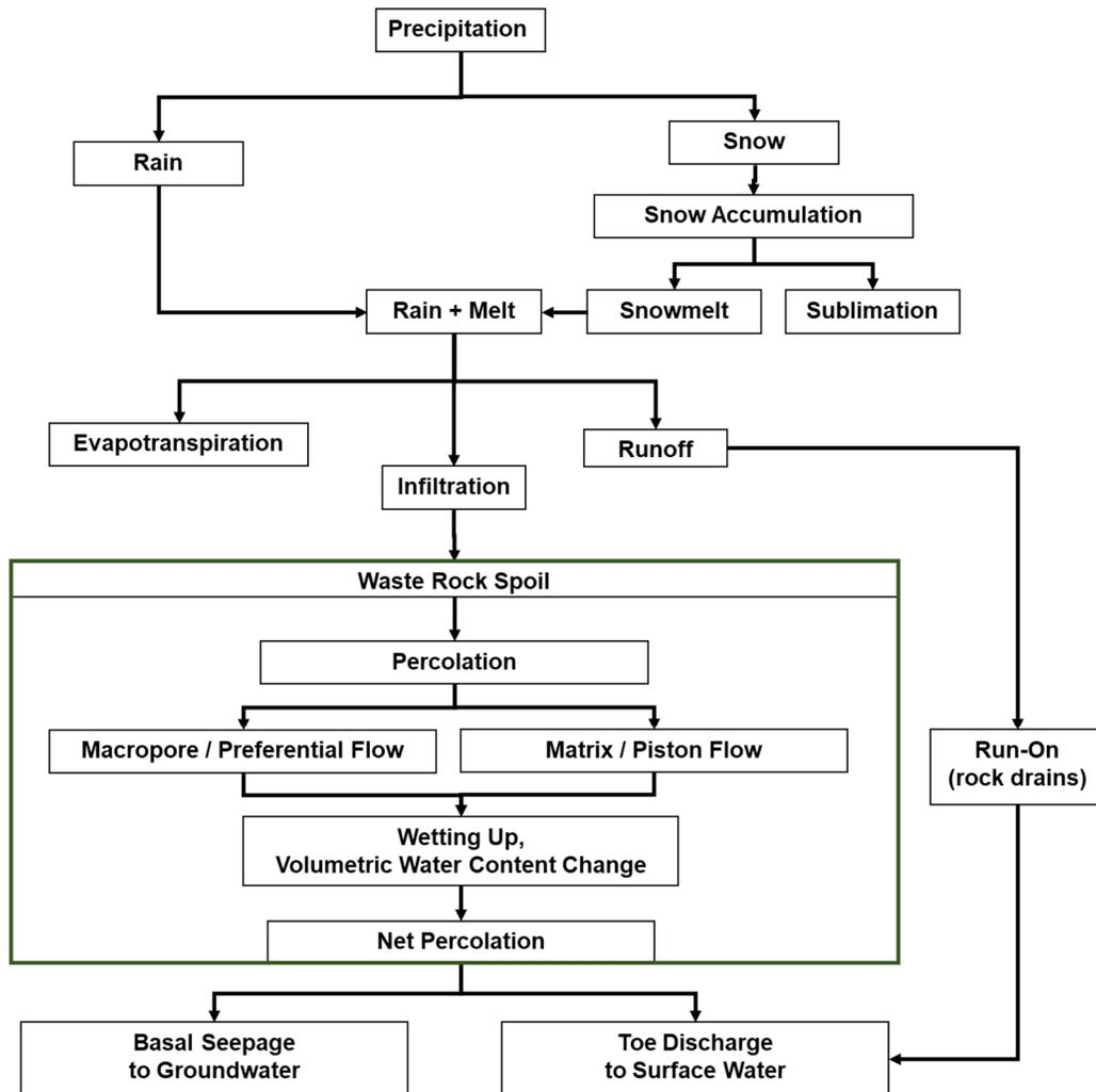
Figure 2-1: Waste Rock Spoil Conceptual Flow Model
