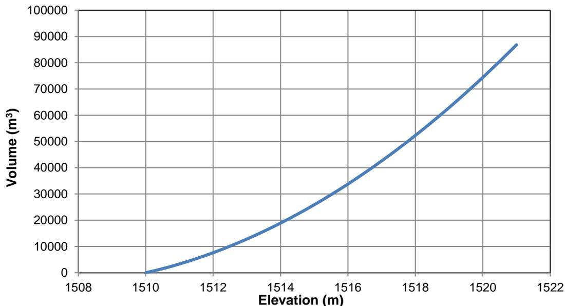
**Figure 3-6: Volume-Elevation Curve for Sediment Ponds**
