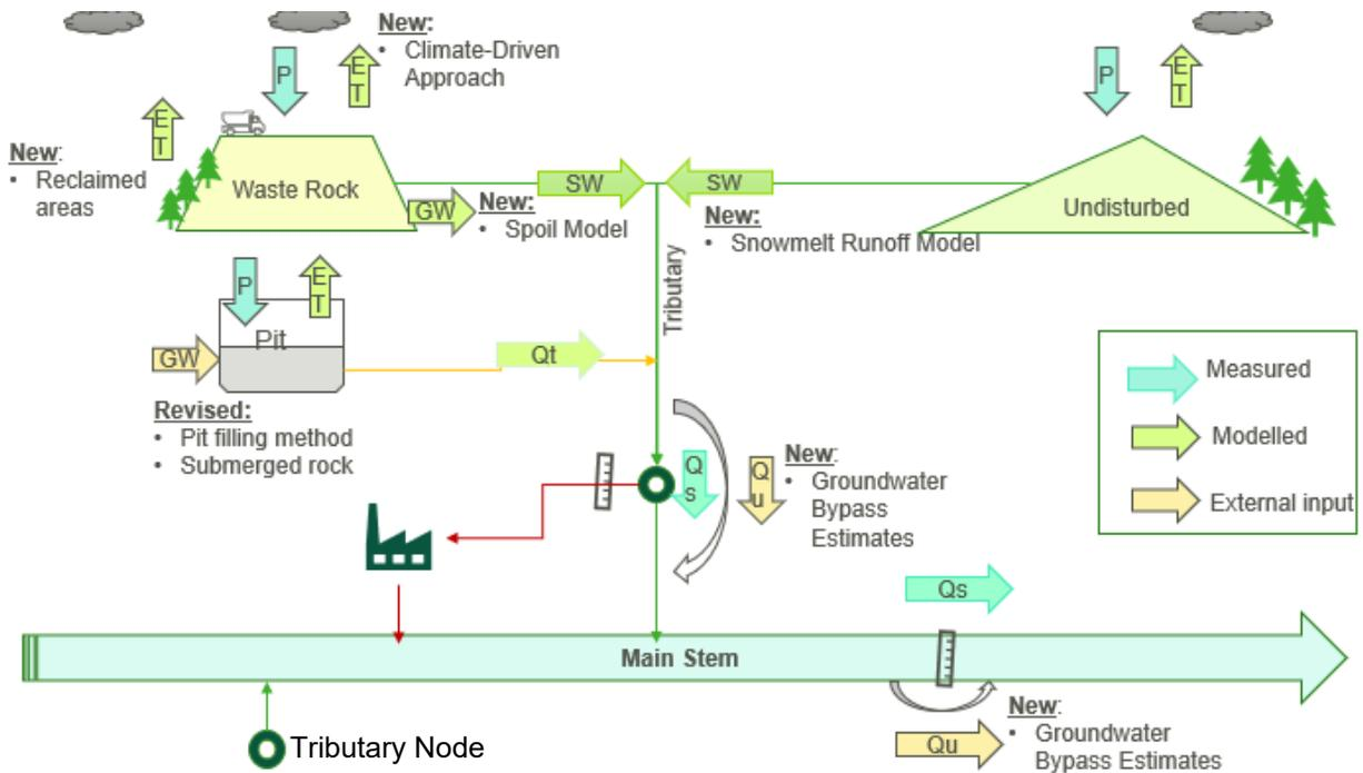
$Q_t$  = Total Flow;  $Q_s$  = Surface Flow,  $Q_u$  = Subsurface Flow, P = Precipitation, ET = Evapotranspiration, GW = Groundwater, SW = Surface Water
