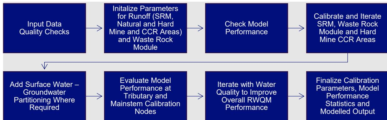
Figure 6-3: Calibration Process for the Flow Component of the 2020 RWQM
