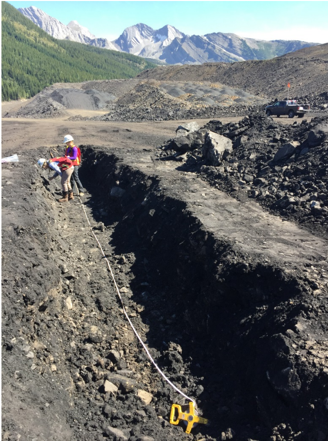
Figure 9. Free Dumped Waste Rock (Background) and Compacted Traffic Surface (Foreground) at Coal Mountain Operations.
