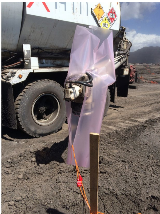
Figure 12. Example of Liner in a Dry Hole Prepared for ANFO Loading. Source: Teck.
