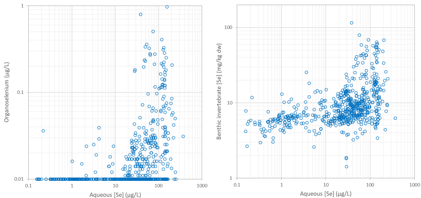
Figure 6. Collinearity of organoselenium (left) and benthic invertebrate selenium (right) with total aqueous selenium
